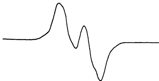
Fig. 2 EPR spectrum of irradiated 2a in the solid state. Measurement conditions: field, 3360 ± 50 G; modulation, 2 GHz; amplitude, 2.5 × 10.
